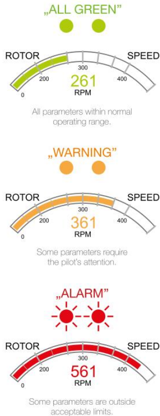
Fig. 7. The idea of flight parameter status information
