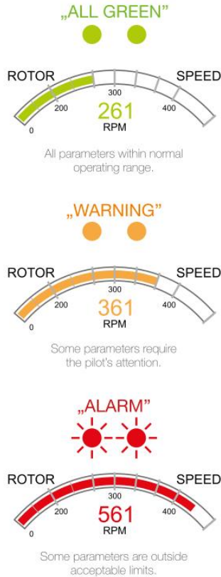
Fig. 7. The idea of flight parameter status information
